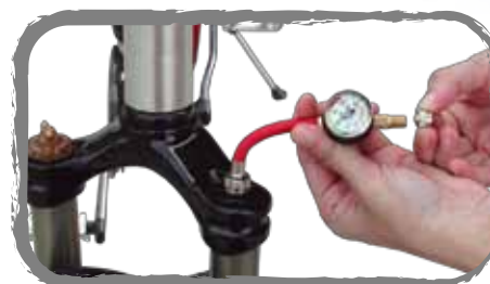
Adjust the pressure by cap
