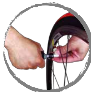
Control the flow of Co2 by turn on or turn off the Co2 cartridge.
